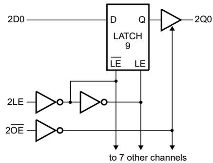
Fig. 3. Logic diagram
